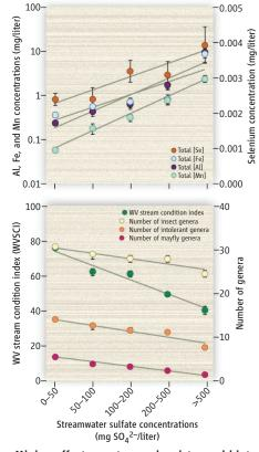
Mining effects on stream chemistry and biota. Sulfate concentrations reflect amount of mining in watershed. (Top) Average concentrations of manganese, iron, aluminum, and selenium. (Bottom) Stream invertebrate community metrics in relation to sulfate concentrations for 1058 WV streams (methods in table S2). Regressions all statistically significant (table S3).
