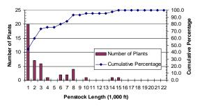
Figure 7. Number of small hydroelectric plants in the Pacific Northwest Region by penstock length interval and cumulative percentage of plants having penstocks of a given length or shorter.
