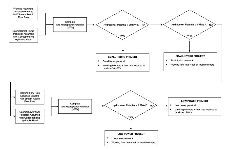
Figure 9. Logic for determining whether a water energy resource site should be developed as a low power or small hydro project using development criteria thereby establishing working flow rate, penstock length, working hydraulic head, and hydropower potential.
