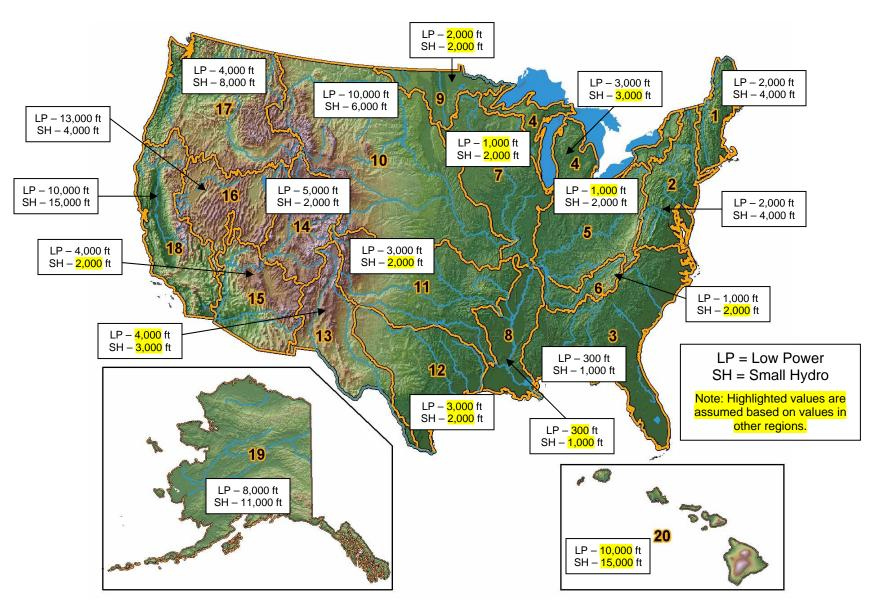
Figure 8. Penstock length upper limits for low power and small hydro plants in 20 U.S. hydrologic regions.
