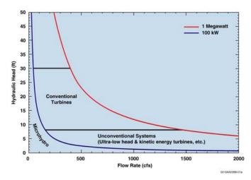
The power and technology classes into which feasible potential projects have been divided based on their hydropower potential and working hydraulic head:
