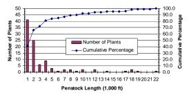
Figure 5. Number of low power hydroelectric plants in the Pacific Northwest Region by penstock length interval and cumulative percentage of plants having penstocks of a given length or shorter.
