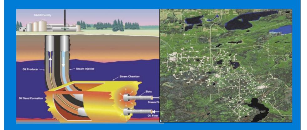
Over 80% of the bitumen can only be extracted 'in situ' whereby high-pressure steam is injected to remove the bitumen from the sand.
