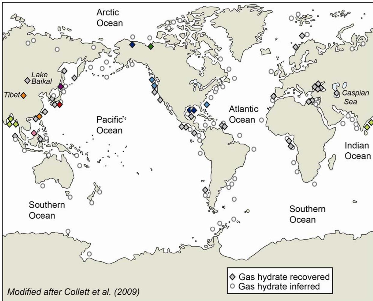
Figure 2. Global map of recovered and inferred gas hydrates, modified from Collett et al. (2009). The color coding refers to drilling programs highlighted in the gas hydrates research timeline shown in Figure 5. This map includes gas hydrates recovered from both shallow depths, which are generally not considered relevant for resource studies, and greater depths. For full discussion see Ruppel et al. (2011).
