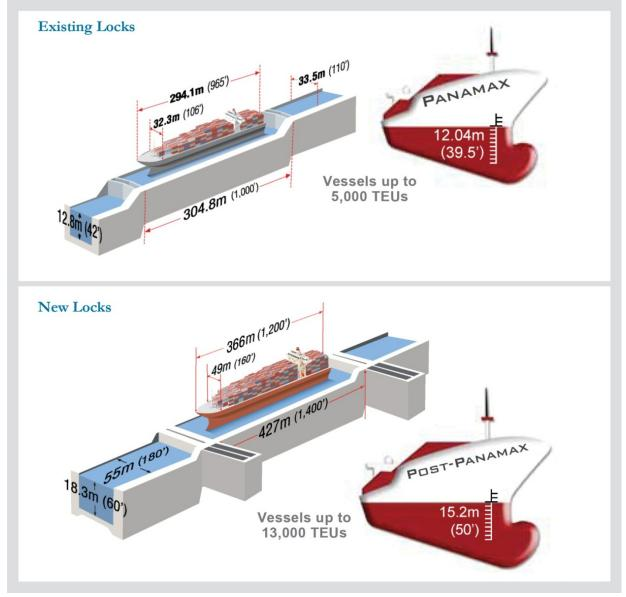
Figure 2. LOCK CONFIGURATIONS FOR EXISTING AND EXPANDED CANAL
